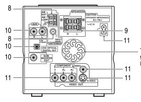
These holes discharge heat generated inside the unit. Do not cover up these holes.
